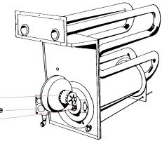
Drum and Tube Heat Exchanger
